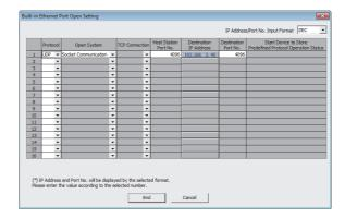
• For "Ethernet Conf.", drag and drop "UDP Connection Module" from "Module List" to the left side on the window. Set the port numbers and IP address as mentioned below.
