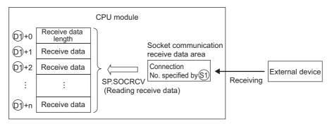
The result of the SP.SOCRCV instruction can be checked with the completion device @+0 and @+1.
