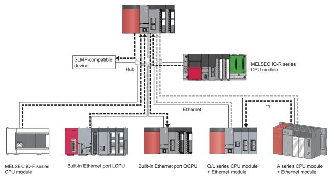
\*1 Device data are communicated between the CPU modules where parameters are not set by relaying the device data via a CPU module where parameters are set.
