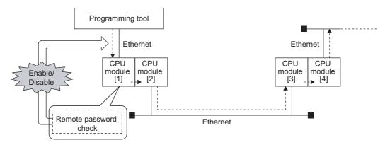
While a remote password is set for all CPU modules, the remote password set for CPU module [1] can be unlocked so that the relay station CPU modules can be accessed without password checking.
