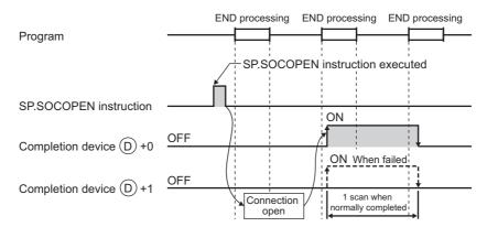
A connection with no parameters (no protocol is specified) can be opened. In this case, specify 8000<sub>H</sub> for \$2+0 and configure open settings in \$2+2 to \$2+9.
