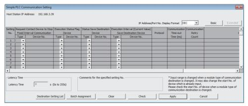
Simple PLC Communication Setting consists of Base Setting (essential) and Extended Setting (optional). To switch the window, use the [Basic] and [Extended] button on the top right of the window.
