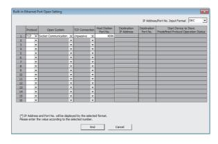
• For "Ethernet Conf.", drag and drop "Unpassive Connection Module" or "Fullpassive Connection Module" from "Module List" to the left side on the window. Set the port numbers and IP address as mentioned below.
