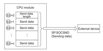
The result of the SP.SOCSND instruction can be checked with the completion device, ①+0 and ①+1.
