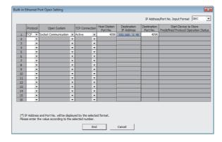
• For "Ethernet Conf.", drag and drop "Active Connection Module" from "Module List" to the left side on the window. Set the port numbers and IP address as mentioned below.
